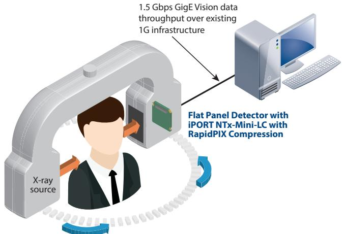
Pleora's patented RapidPIX lossless compression converts video data into GigE Vision compliant packets that are transmitted at up to 1.5 Gbps throughput rates over existing 1 Gbps infrastructure. The compression technique, integrated into Pleora's iPORT NTx-Mini-LC platform, is optimized to ensure original and post-compression data are identical while supporting ultra-low latency performance for mission-critical applications.
