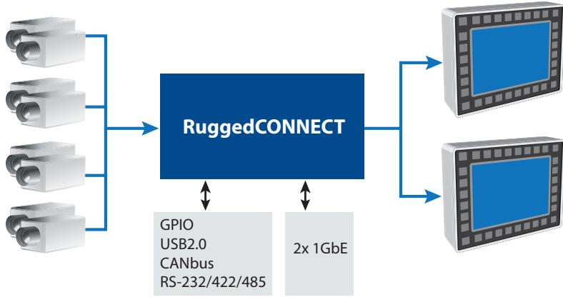
**All-in-one rugged Smart Video Switcher for sensor capture, streaming, processing, and display**
