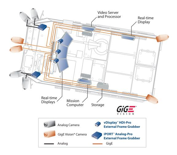
Figure 1: Video converted to GigE Vision by an external frame grabber and streamed over the multicast Ethernet network to displays and processing equipment at various points within the vehicle.
