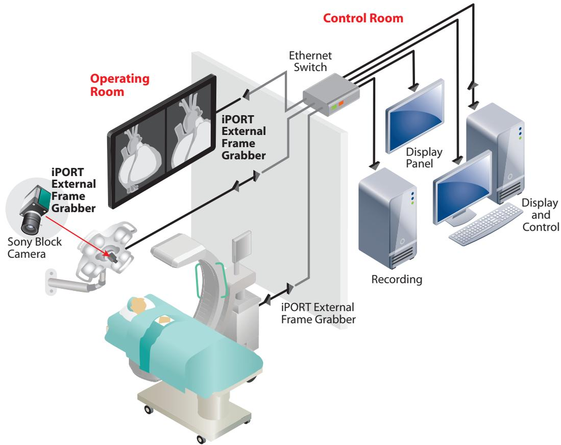
Diagram 1: Images from an X-ray detector and lamp-head camera are converted to GigE Vision and multicast to display panels in the operating room and computing platforms used for image processing, storage, and monitoring.
