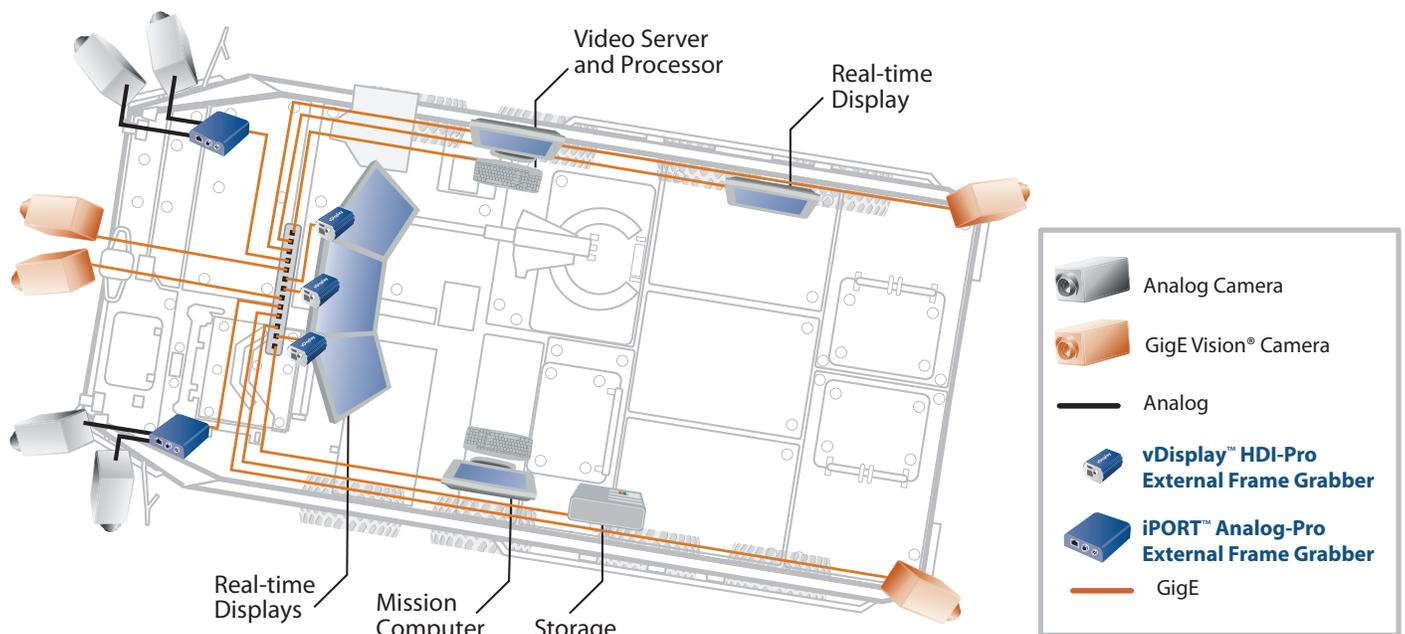
Figure 1: Video is converted to GigE Vision by an external frame grabber and streamed over the multicast Ethernet network to displays and processing equipment at various points within the vehicle.
