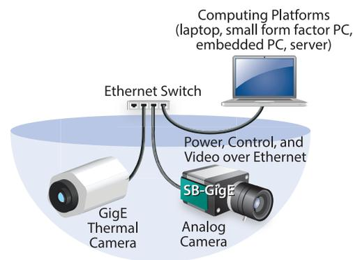
Figure 2: Images from an analog camera are converted into GigE Vision video and blended with video from a native GigE Vision thermal camera.
